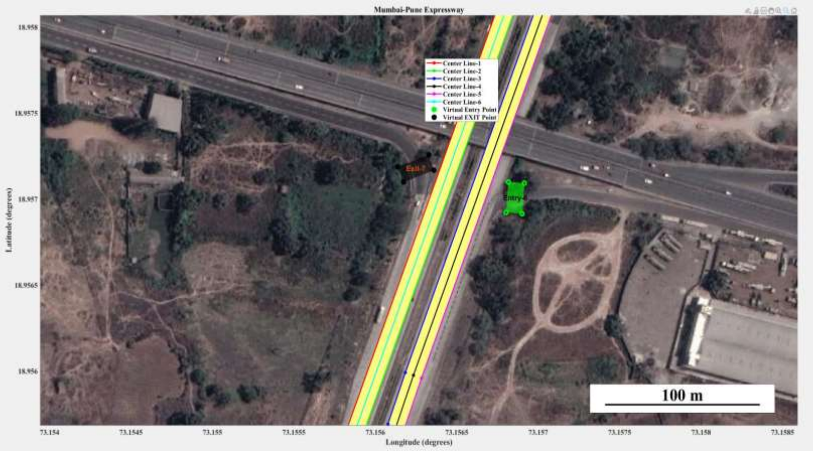
Example virtual gantry definition at the intersection of the toll-able and non-tollable roads
