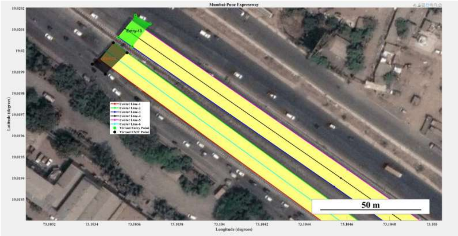
Example virtual gantry definition at the entrance (in green) or exit (in black) of the toll-able road and also the polygon data (in yellow)
